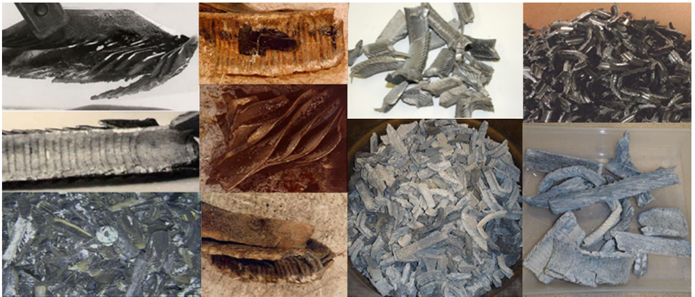
Figure 1: Active swarf on the left and inactive swarf on the right.
