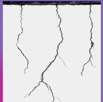
5mm deep CO 2 SCC defects
